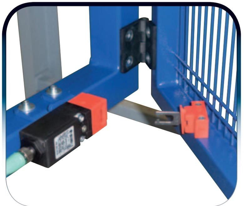
Machine stop safety device for guards opened. Cycle start and automatic operations are only possible when all machine guards are closed.
